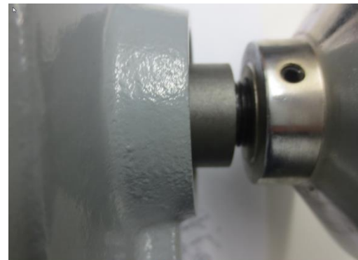
Put distance sleeve and screw on handwheel
