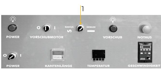
The mode selector switch (1) selects the mode of operation:
