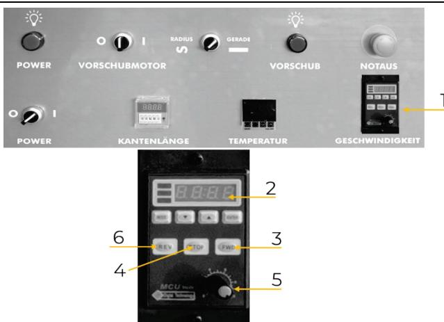
The feed control unit (1) is used to set/display the feed speed (motor speed drive roller) and activate the motor start.
