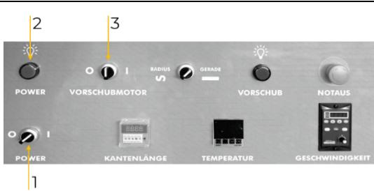
Turn the main switch (1) to position ON (I). The control lamp (2) lights up.
