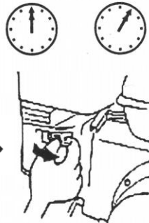
Let the machine run in idle run for 5 Minutes – then Choke back
