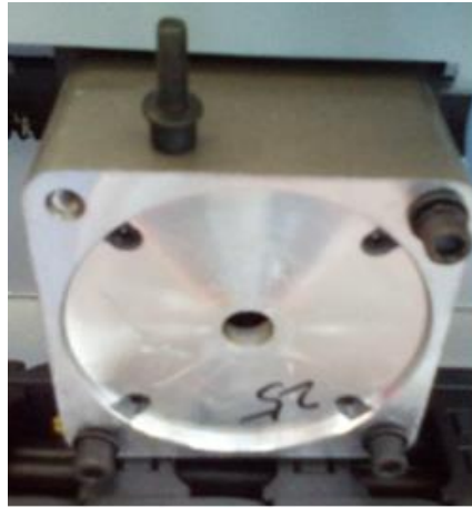
2. Travelmotor Mount with 4 screws
