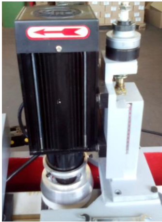
1. Mainmotor: Mount with 4 screws
