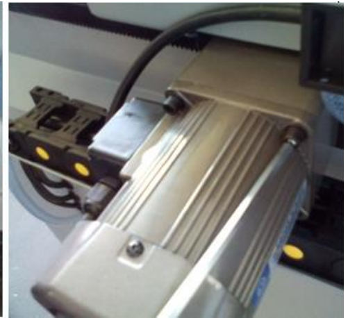
2. Travelmotor Mount with 4 screws
