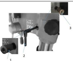
5. Mounting machine head fixation lever
