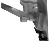
Mounting hand crank for working table
