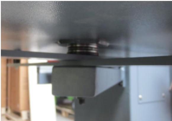
One of the two thrust bearings put centrally on the flat iron.
